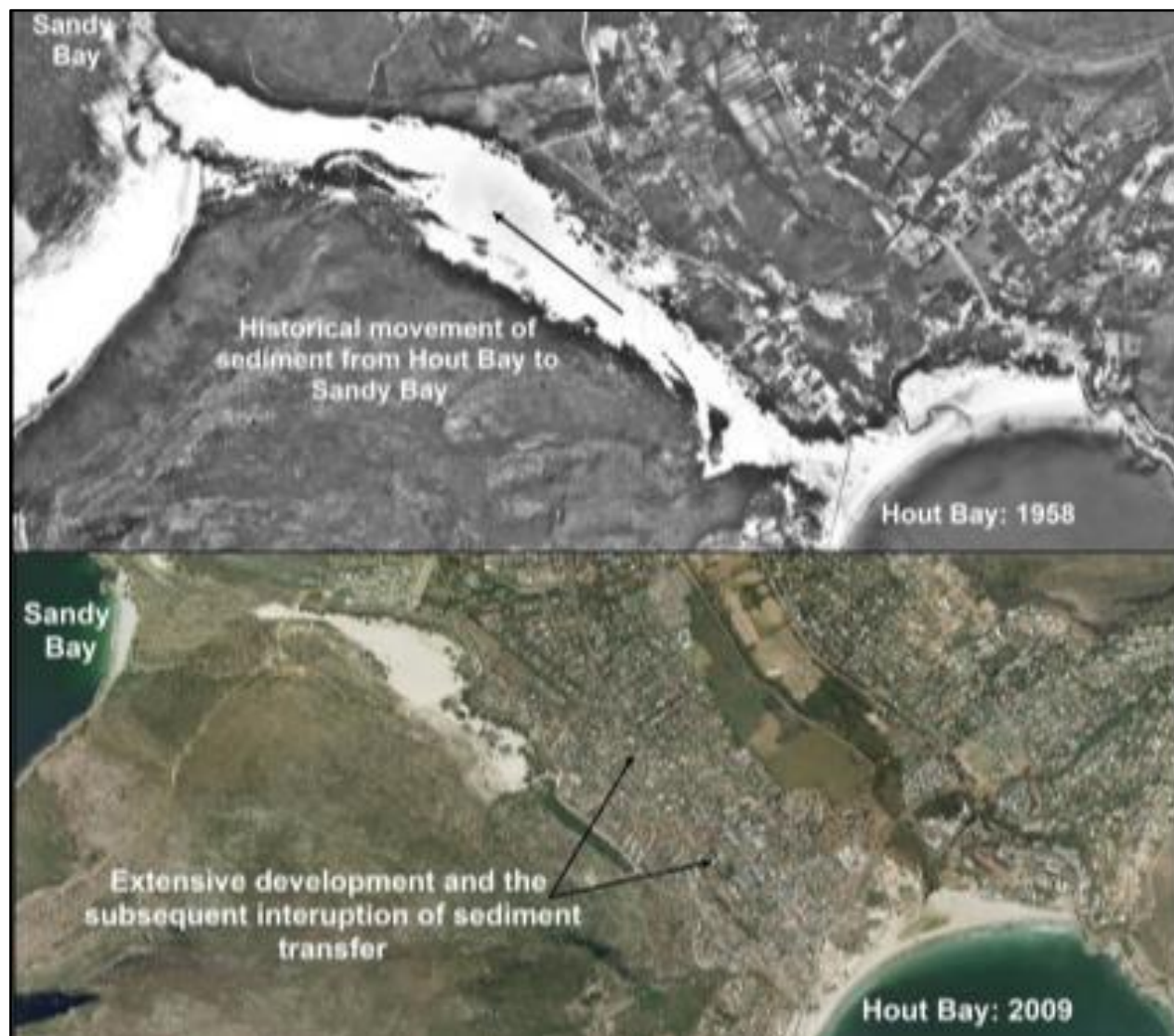
Figure 2: sediment by-pass and dune systems that have been severely altered by coastal development.
